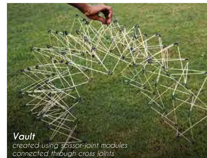
Vault created using basic scissor-joint modules
