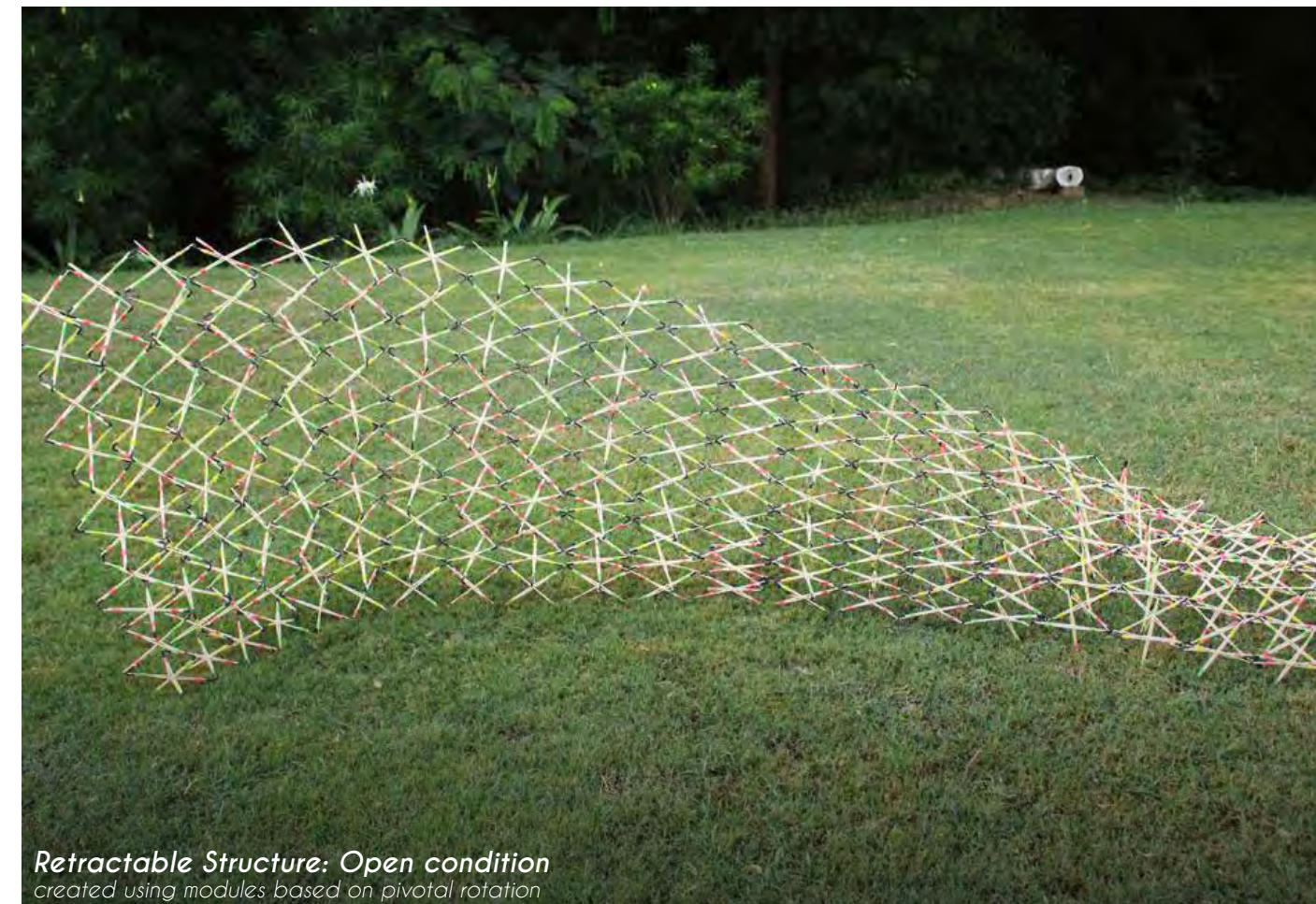
Vault created using scissor-joint modules connected through cross joints
